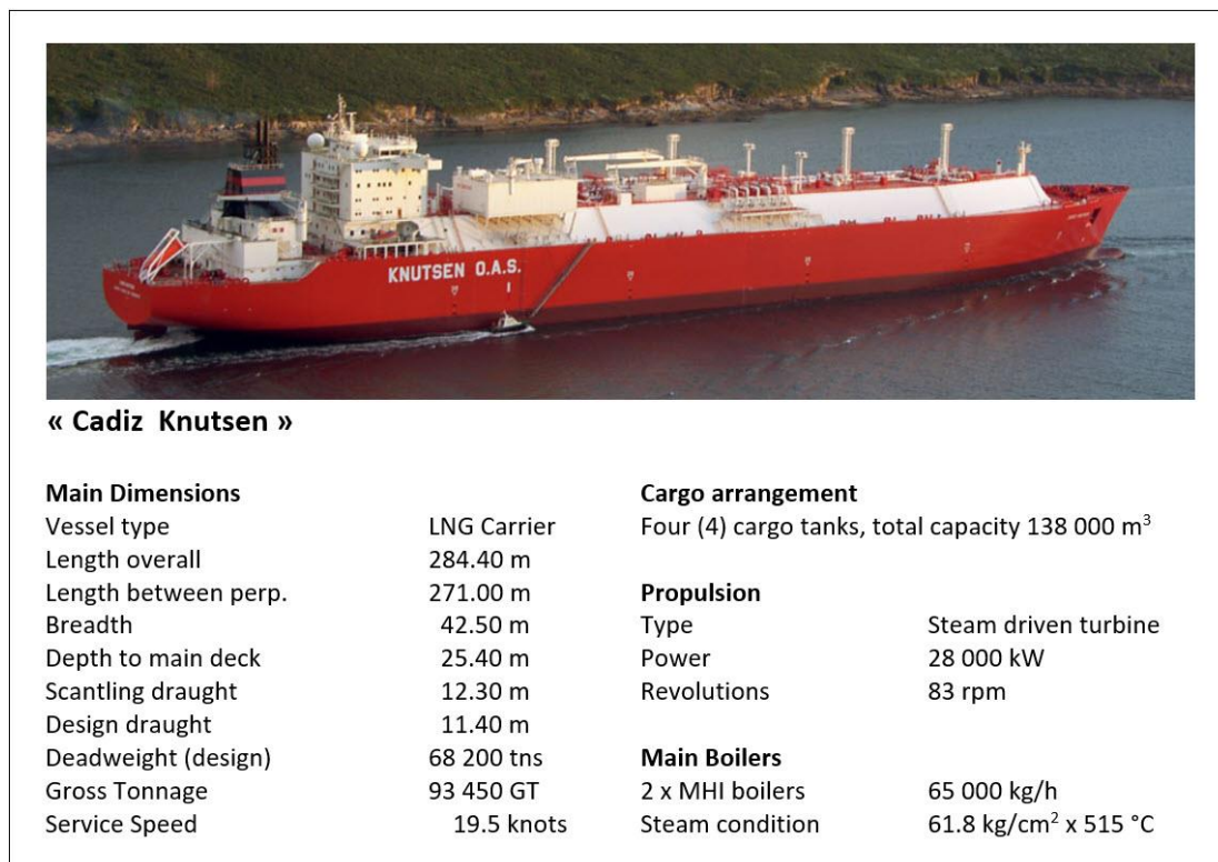
FIGURE 1: TYPICAL LNG CARRIER BEING CONSIDERED FOR CONVERSION TO NUCLEAR PROPULSION. SOURCE: KNUTSEN OAS.
